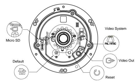
**Video System:** NTSC / PAL system switch. Default is NTSC. Use a suitable small tool to operate the switch.
