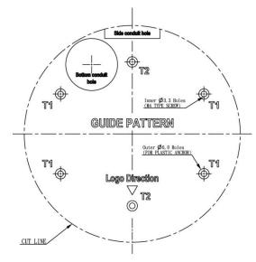
Method 3: To surface mount using junction box
