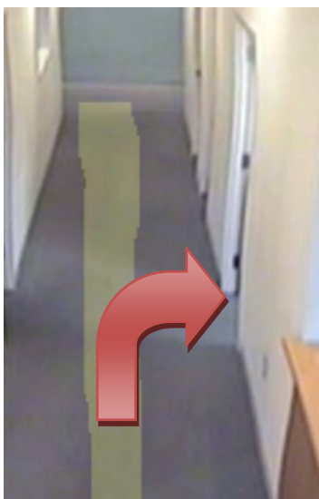
Fig. 3— If a person started at the bottom of the path and then turned right into the first office door, the person would not be detected because the person did not cover the majority of the yellow ROI drawn on the floor.
