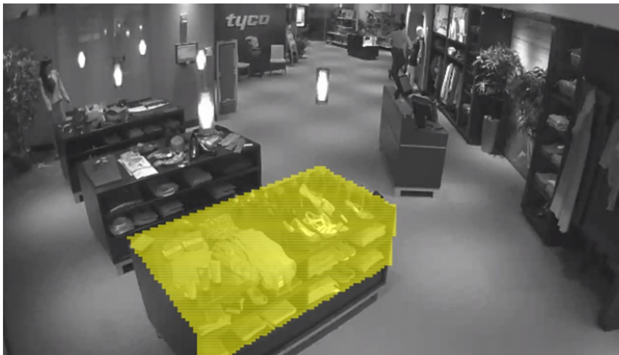
Fig. 8— When using Abandoned/Removed to monitor assets it is best to draw an ROI closely fitting the display fixture. When you do this, the Amount Changed matches the assets taken. Use a higher Overlap so that changes near the fixture are ignored.
